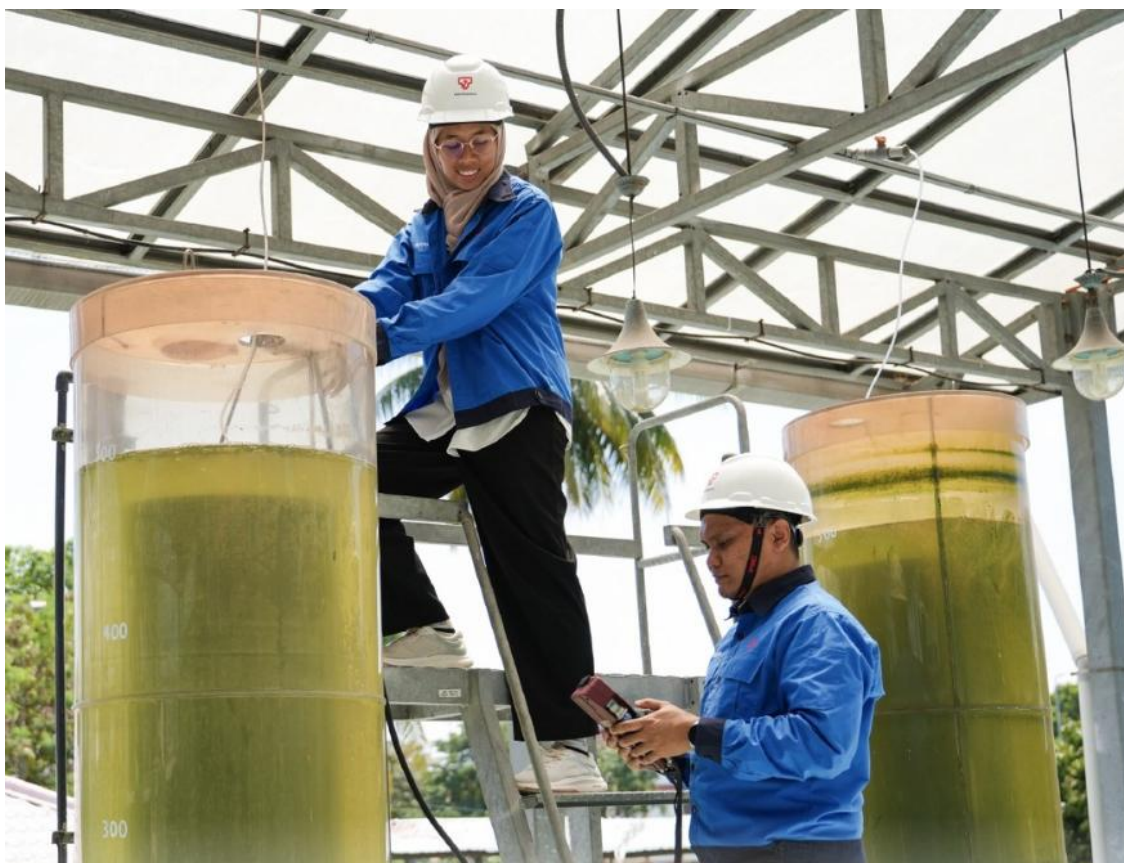
Figure 6: Photobioreactor system for Bio-CCU [37]
