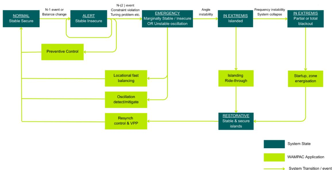
**Figure 11** Typical WAMPAC Operation Diagram in Various System States [20]
