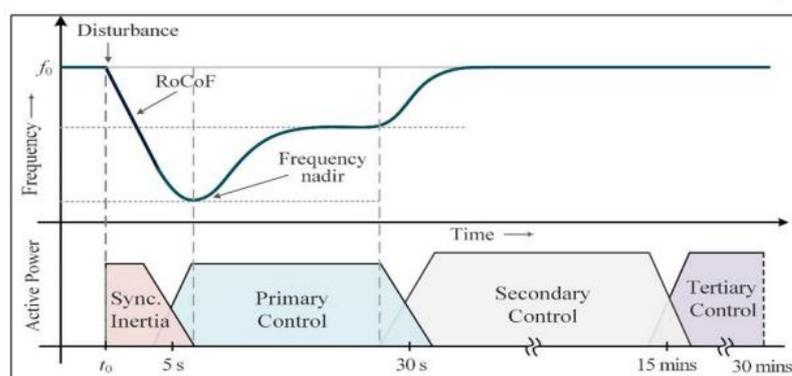
**Figure 7** Frequency Response and Control Timeline Following a Disturbance [18]
