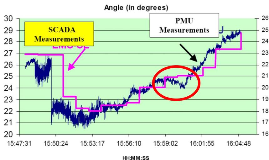
**Figure 12** SCADA vs. PMU Measurements [23]
