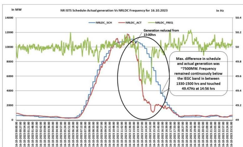
**Figure 4** Impact of Cloud-Shading on Solar Power Generation and System Frequency in October 2023 [10]
