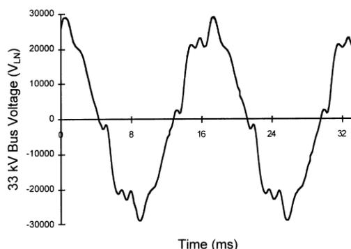
**Figure 5** Illustration of Harmonic Distortion on Voltage Waveform [12]
