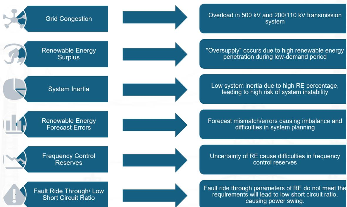
**Figure 6** Operational Challenges of High VRE Penetration in Viet Nam's Power System [16]
