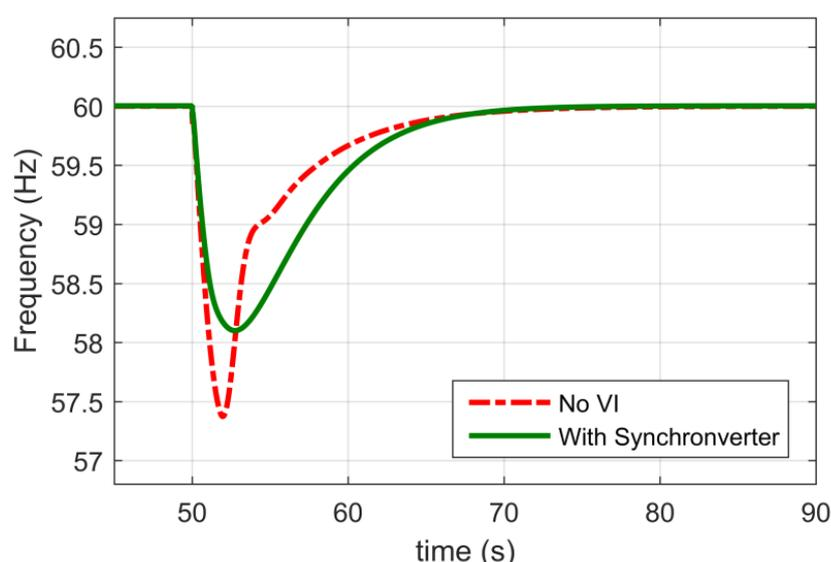
**Figure 3** Lab Simulation of Synchronverter Implementation on Frequency Drop [9]
