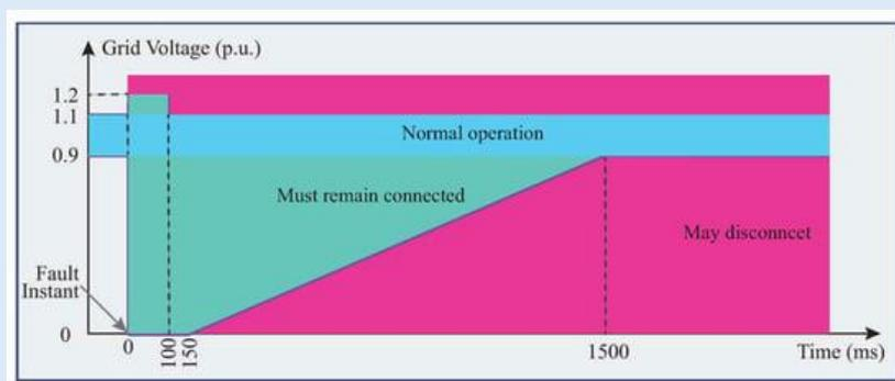
**Figure 8** Fault Ride Through Diagram [24]
