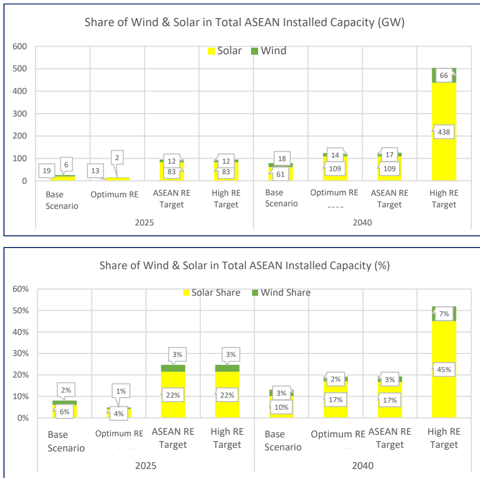
Figure 3-24: Comparison of Share of VRE Capacity in 2025 and 2040 for All Scenarios – ASEAN Region
